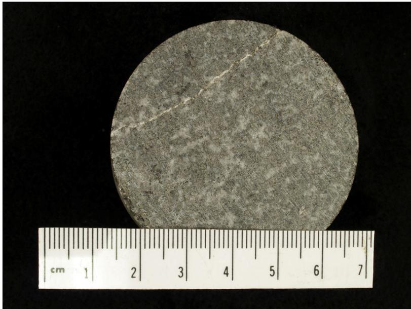
**Figure 1** – Image of sawn core from which thin section was made. Rock displays a medium- to coarse texture consisting predominately of intergrown pyroxene (dark) and plagioclase (light) phases. Note thin vein of calcite cutting across upper left part of sawn core. Greenish tints are the result of alteration to amphibole and chlorite. Thin section cut from depth of 3.95'.
