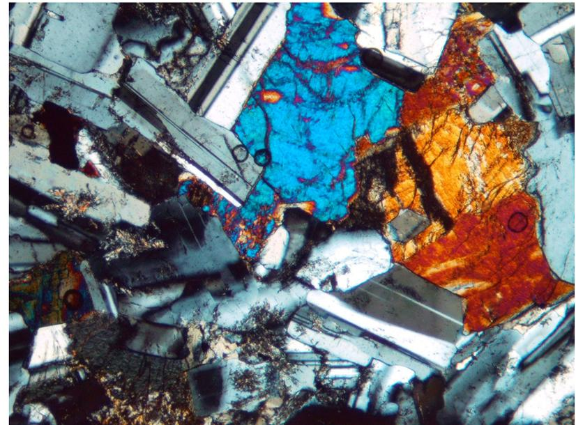
**Figure 2** - Photomicrograph showing interstitial growth of twinned clinopyroxenes (large crystals of augite with blue and orange interference colors) grown in angular areas between zoned and twinned lath-like crystals of plagioclase feldspar. The feldspar is slightly weathered, internally altered to clay and sericite in some crystals. Note the triangular arrangement of feldspar crystals, typical of diabasic texture.
