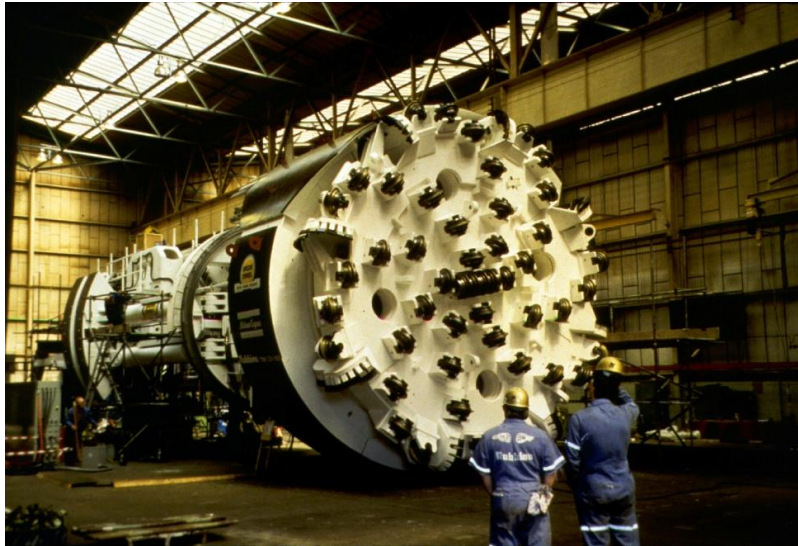
Figure 2 - The front cutterhead and thrust assembly (business-end = 84' length and 23' diameter) of the Tunnel Boring Machine that formerly operated beneath western Queens. With a total length of nearly 300', the complete machine excavates, processes, and removes the rock chipped by the cutters. The cutterhead rotates against the raw rock face with thrust applied hydraulically by mechanical contact from behind against the sides of the bored tunnel. The TBM holed-through beneath Long Island City in October 1999 after three years of nearly continuous subsurface mining.
